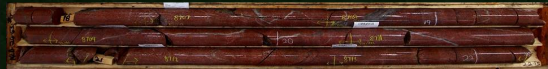
KLD26-63 17.8m to 22.15 m highly altered syenite
