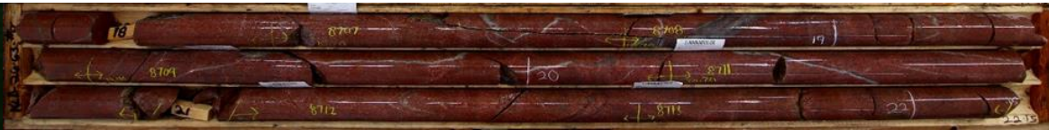
KLD26-63 17.8m to 22.15m highly altered syenite.
