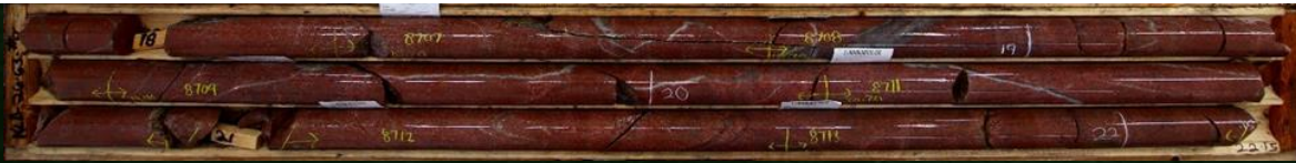
KLD26-63 17.8m to 22.15m highly altered syenite.
